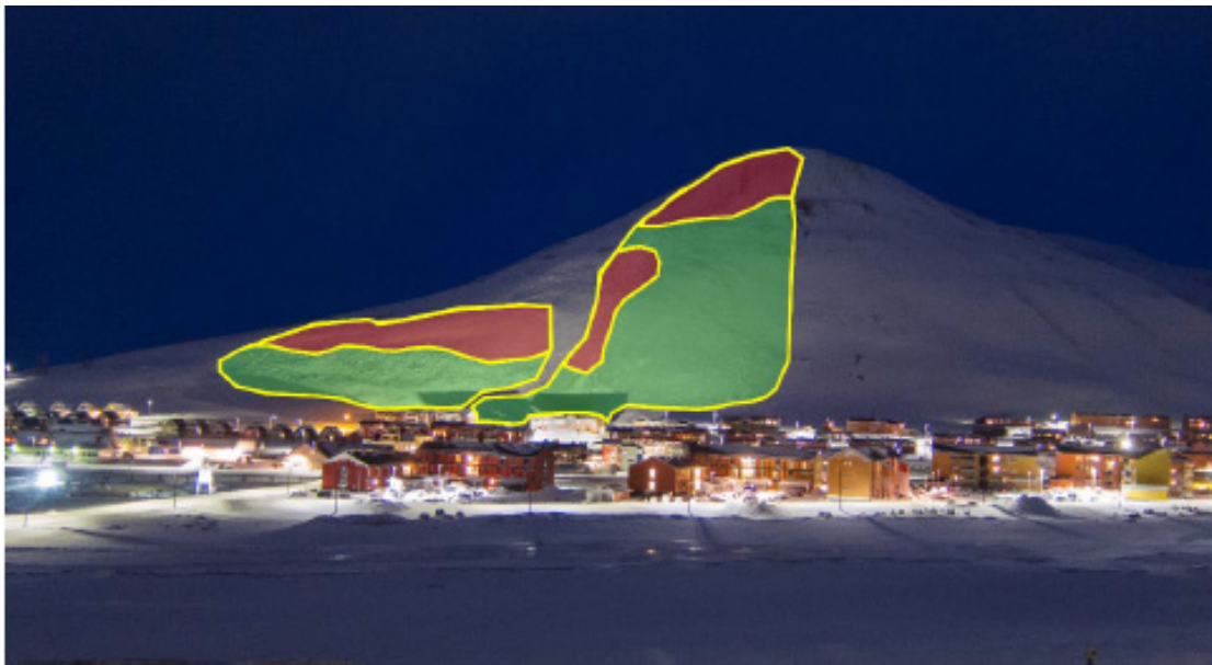
Photo 6.1: Illustration of 2017 avalanche with assumed release areas (red) and runout area (green) from NVE (2017).
